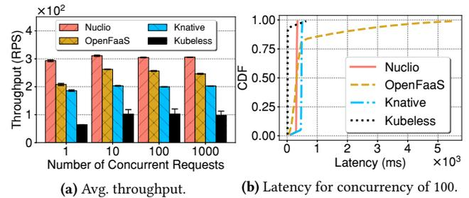
Figure 7. Throughput & latency of ‘http-workload’ function across different serverless platforms at different concurrency levels.
