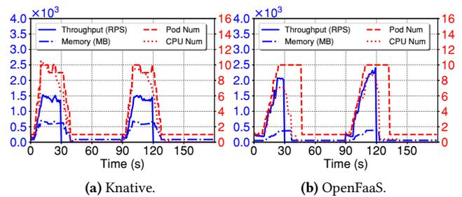
Figure 12. Auto-scaling with bursty workload.
