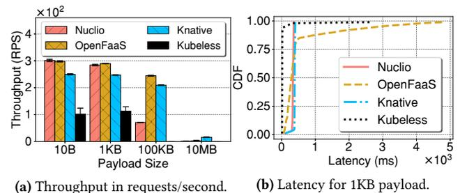
Figure 8. Throughput & latency of ‘http-workload’ function with different payload sizes for different serverless platforms.
