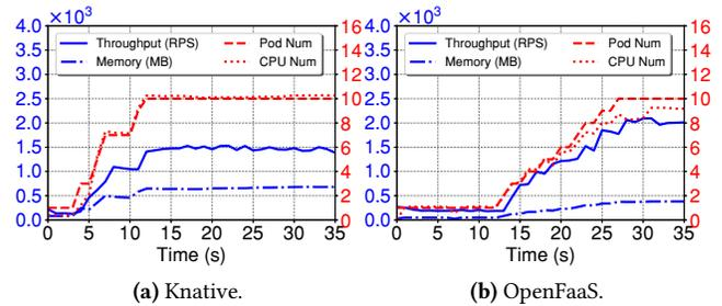
Figure 11. Auto-scaling with steady workload.
