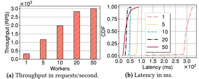
**Figure 3.** Throughput and latency for different number of workers within one Nuclio function pod (100 concurrent requests).
