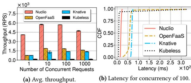
Figure 6. Throughput and latency of ‘hello-world’ function.
