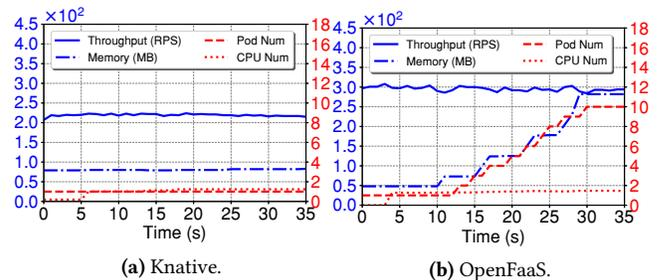
Figure 13. Auto-scaling issues with Knative and OpenFaaS.
