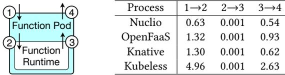
Figure 10. Latency breakdown (ms) parts of serverless execution.
